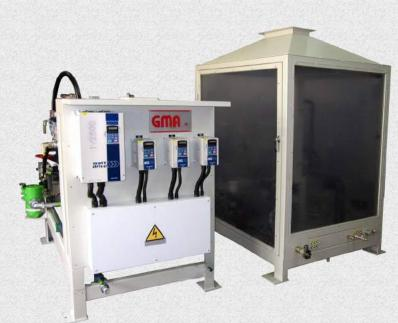
Rim Polymer's GMA branded cyclopentane metering group consists of various components which contributes to its favourable output. A cyclopentane metering pump which is simple in design yet versatile in use. This is coupled with a fail-safe valve which is installed at the suction line of the metering pump and an AC inverter motor which has closed-loop controlled function.
