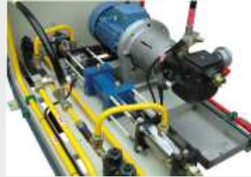
High pressure metering pump with magnetic coupling
