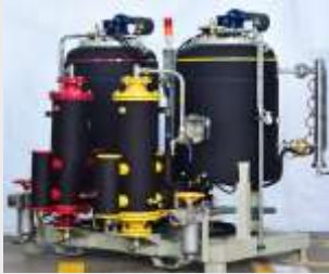
Jacketed Carbon Steel storage tank
